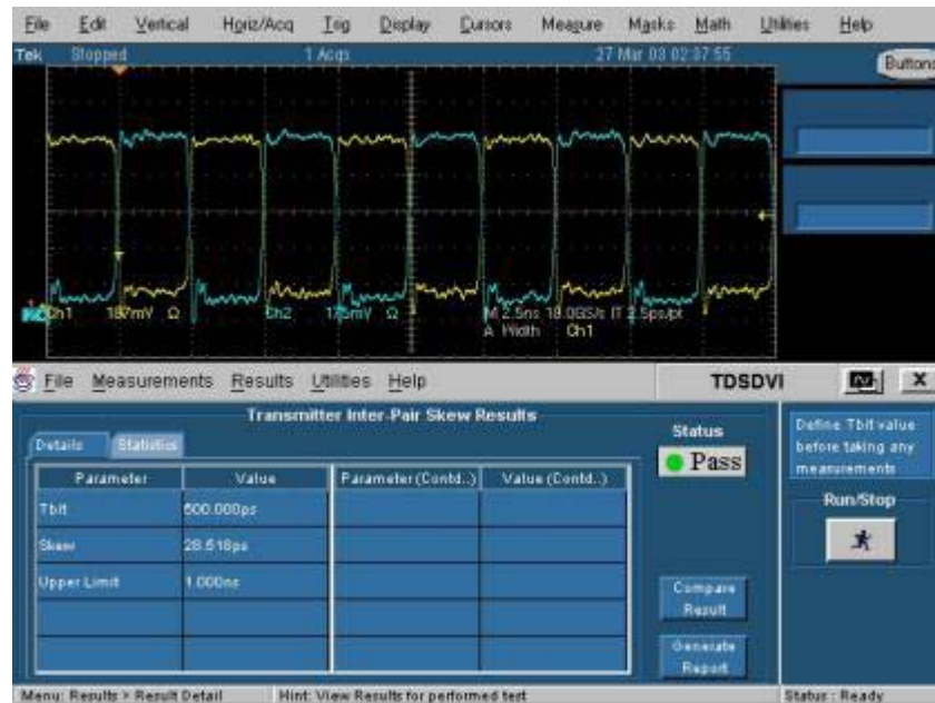
Figure 3-131: Inter-Pair Skew results
