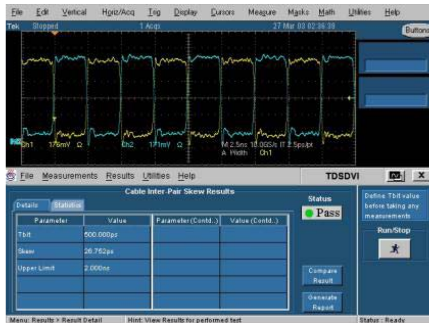
Figure 3-170: Inter-Pair Skew results
