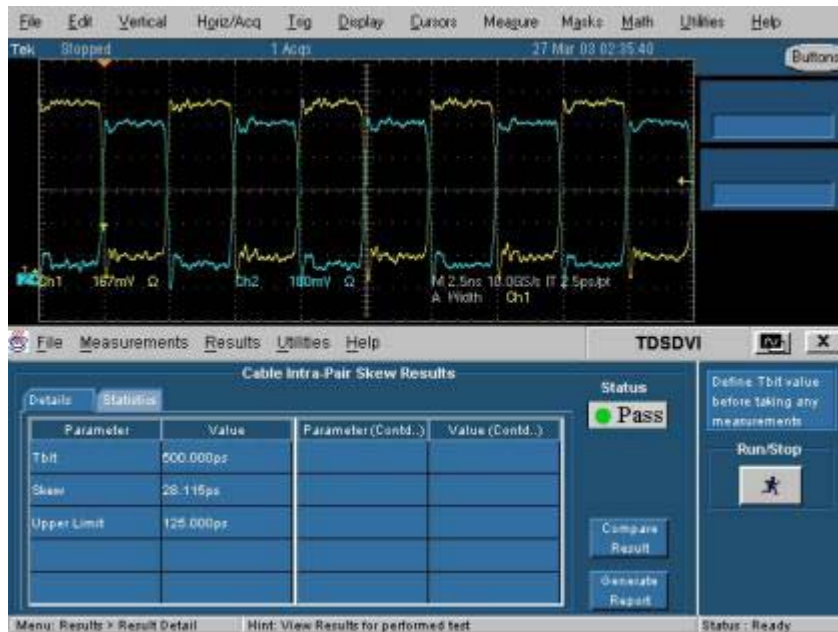
Figure 3-164: Cable Intra-Pair Skew results
